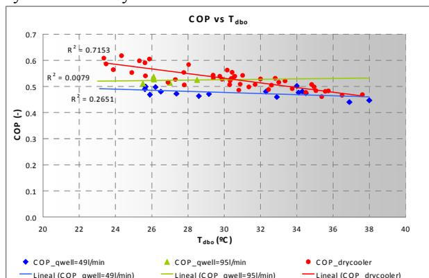
Fig. 8. COP results with the dry cooler and the new geothermal sink
