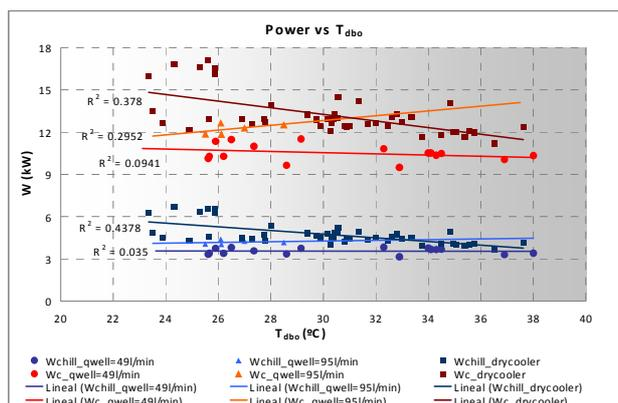
Fig. 7. Chilling capacity and rejected heat power with the dry cooler and the new geothermal sink
