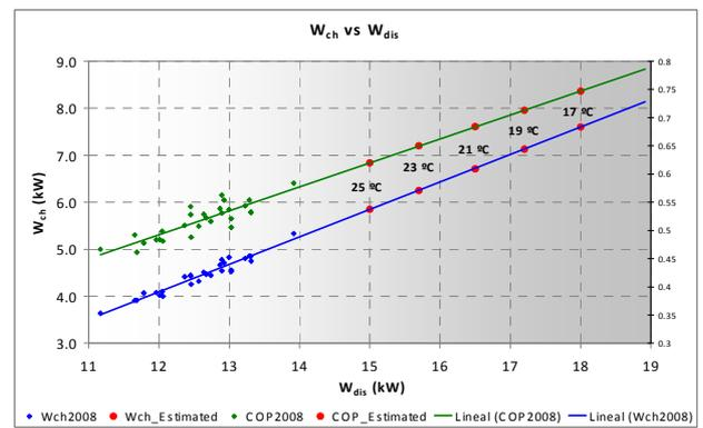
Fig. 5. Chilling power and COP according to cooling capacity and water well temperature
