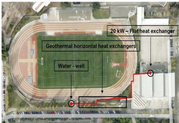
Fig. 1. Situation of the geothermal system
