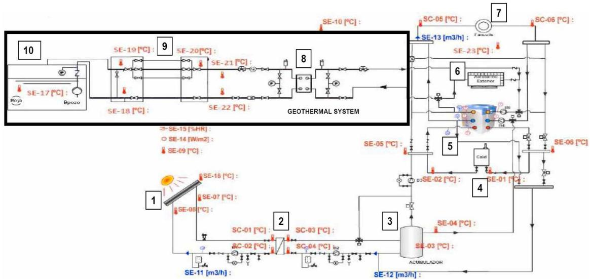
Fig. 2. Scheme of the installation
