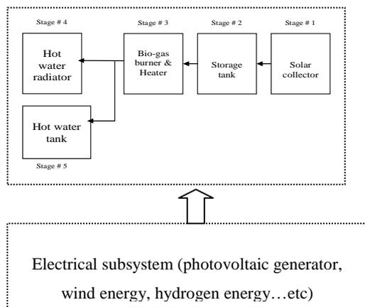
Fig. 1 Block diagram of the global heating system.
