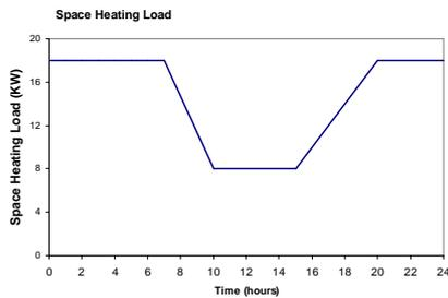
Fig. 3 Space heating load for the hospital building.
