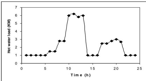
Fig. 5 Hot water heating load in hospital
