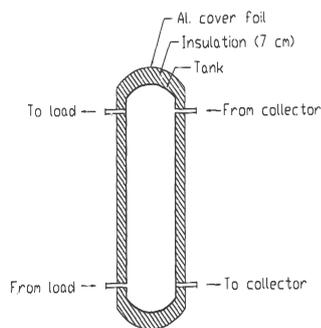
Fig. 8 The storage tank
