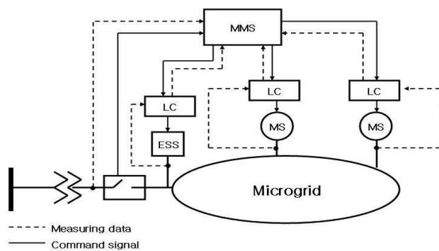
Fig. 1. The hierarchical control structure of microgrid.
