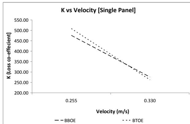
Figure 1: Constant k as a function Velocity [Single Panel]
