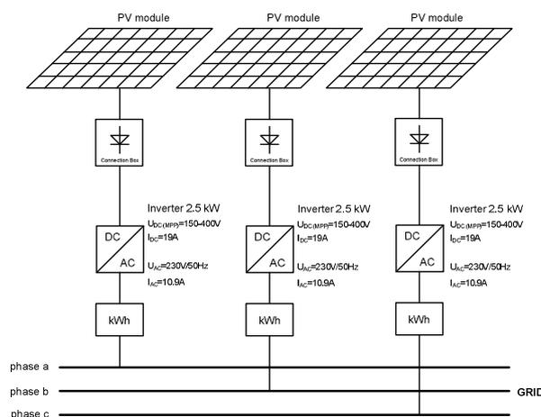
Fig. 1. System block diagram of a photovoltaic system 7,5 kWp installed at University of Maribor.
