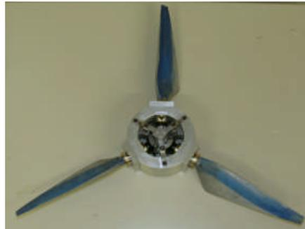
Fig. 1. Model wind turbine with the pitch control mechanism in the hub
