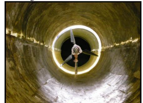
Fig.4. Internal view of the Betz tunnel with model turbine
