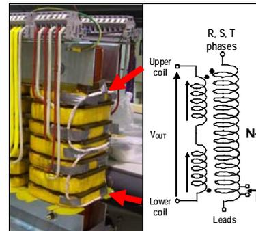
Fig. 3. Air core coils attached to the surface of the transformer windings
