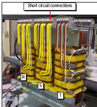
Fig. 1. External appearance of the transformer
