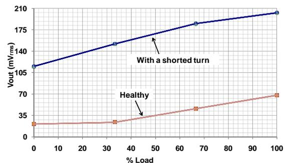
Fig. 4.  $V_{OUT}$  rms value vs. load level in the cases of the healthy transformer and with an interturn short circuit
