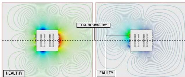
Fig. 2. Leakage flux lines. Left: healthy machine. Right machine with a shorted turn.
