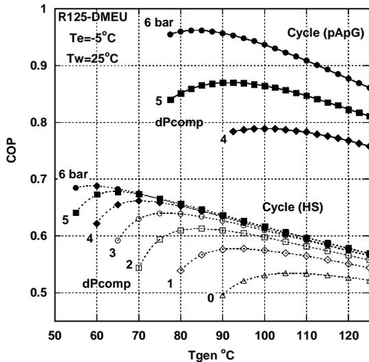
Fig. 3. The calculated COP of hybrid TPL absorption cycle as a function of the generator temperature at various dP with R125-DMEU.
