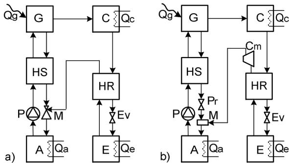
Fig. 1: Single-stage TPL absorption cycle with: a) jet-ejector mixer and b) a compressor and mixing device instead the jet-ejector mixer (cycle HS).
