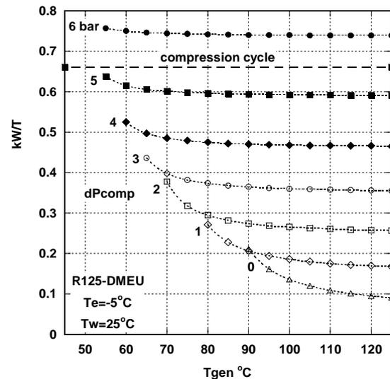
Fig. 6. The calculated kW/T of an isentropic compression cycle and of hybrid TPL absorption cycles as a function of the generator temperature at various dP with R125-DMEU.
