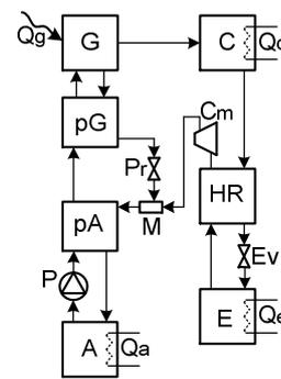
Figure 2: Single-stage TPL absorption/compression cycle with pre-generator - pG, pre-absorber - pA and a compressor and a mixer instead the jet-ejector (cycle pApG).
