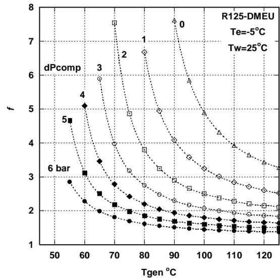
Fig. 5. The calculated circulation ratio  $f$  of hybrid TPL absorption cycles as a function of the generator temperature at various dP with R125-DMEU.
