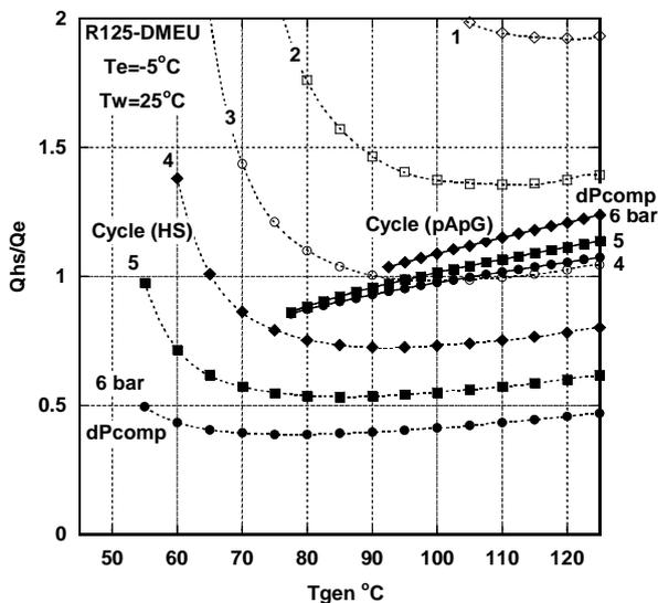
Fig. 4. The calculated  $Q_{hs}/Q_e$  of hybrid TPL absorption cycle as a function of the generator temperature at various dP with R125-DMEU.
