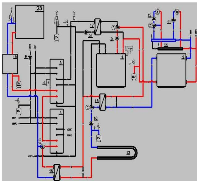
Fig.4. The heat exchange unit. The View of heat carrier flow in the warm period.
