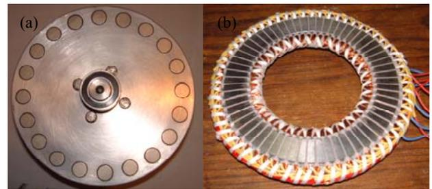
Fig. 9: Generator rotor disk (a) and one stator ring (b).
