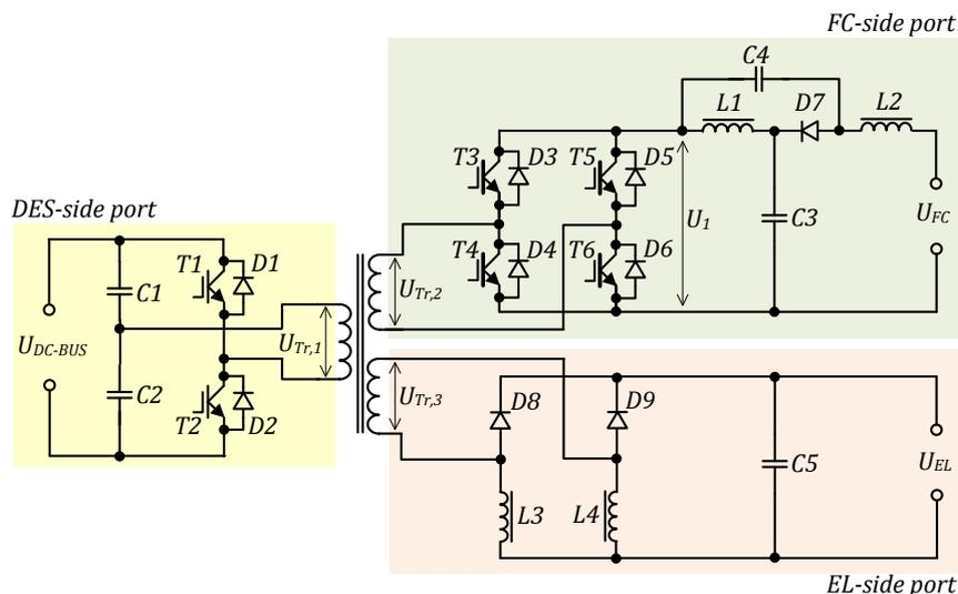
Fig. 3. Power scheme layout of the proposed integrated converter for hydrogen buffer interfacing in DES.
