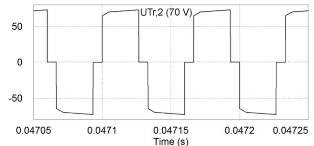
Fig. 9. General operating waveforms of the proposed multiport converter during the FC mode: secondary winding voltage of the isolation transformer ( $U_{Tr,2}$ ).
