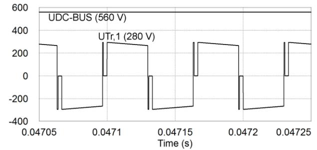
Fig. 6. General operating waveforms of the proposed multiport converter during the EL mode: DC-bus voltage ( $U_{DC-BUS}$ ) and primary winding voltage of the isolation transformer ( $U_{Tr,1}$ ).
