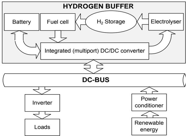
Fig. 2. Proposed structure of the distributed energy system with hydrogen buffer interfaced via multiport converter.
