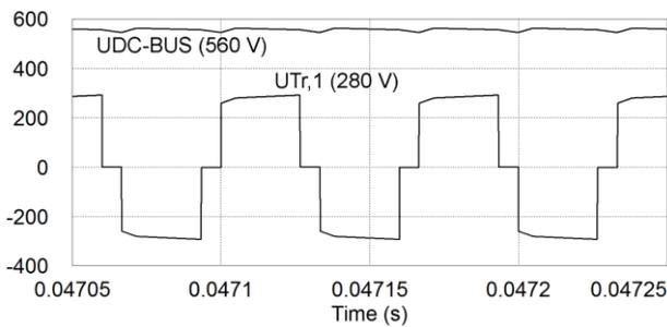
Fig. 10. General operating waveforms of the proposed multiport converter during the FC mode: DC-bus voltage ( $U_{DC-BUS}$ ) and primary winding voltage of the isolation transformer ( $U_{Tr,1}$ ).
