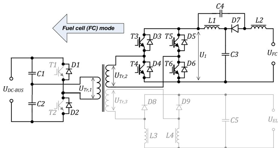
Fig. 5. Power circuit configuration in the fuel cell (FC) mode.
