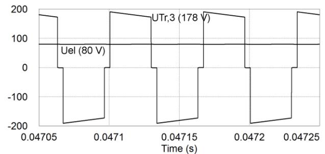
Fig. 7. General operating waveforms of the proposed multiport converter during the EL mode: electrolyser voltage ( $U_{EL}$ ) and tertiary winding voltage of the isolation transformer ( $U_{Tr,3}$ ).
