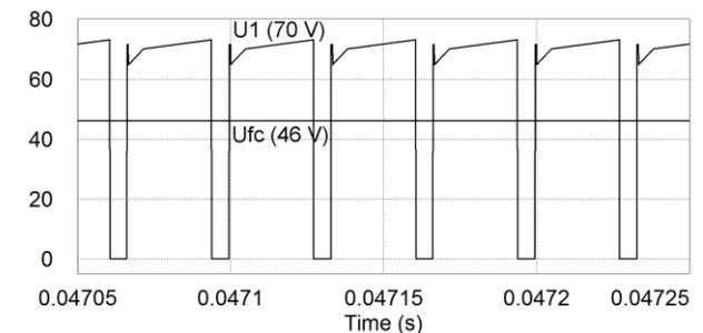
Fig. 8. General operating waveforms of the proposed multiport converter during the FC mode: fuel cell voltage ( $U_{FC}$ ) and intermediate DC-link voltage ( $U_1$ ).
