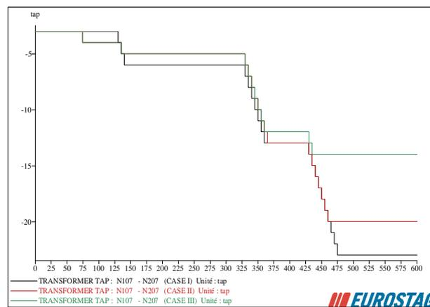
Fig. 12. Under Load Tap Changers position.
