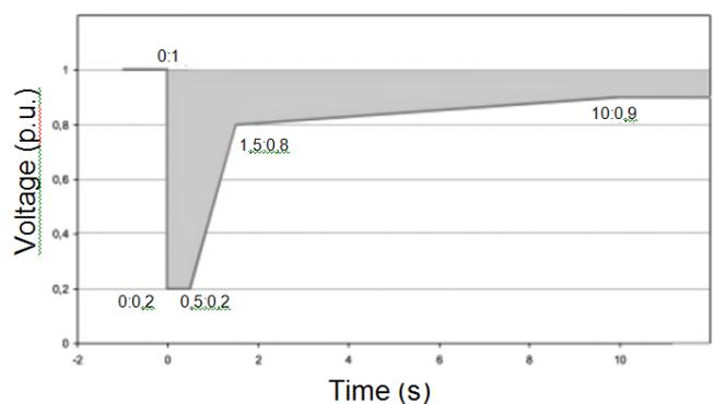
Fig. 3. Requirements of "Fault Ride Through Capability – FRTC" [8].
