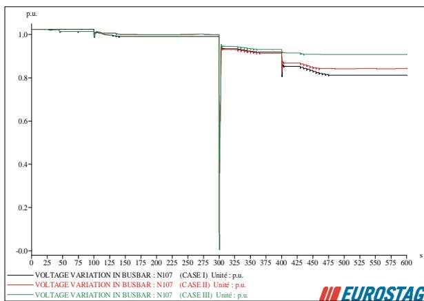
Fig. 10. Voltage variation in busbar 107.
