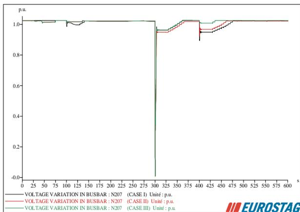
Fig. 11. Voltage variation in busbar 207.
