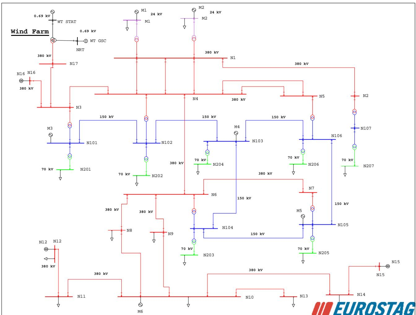
Fig. 4. Cigré test power network single line diagram [9], [10].
