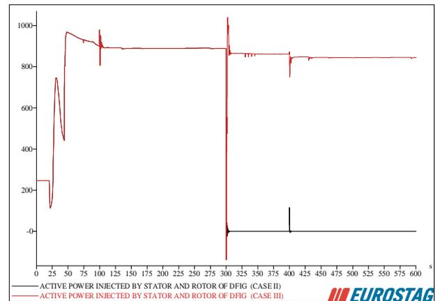
Fig. 8. Active power injected by stator and rotor of DFIG.
