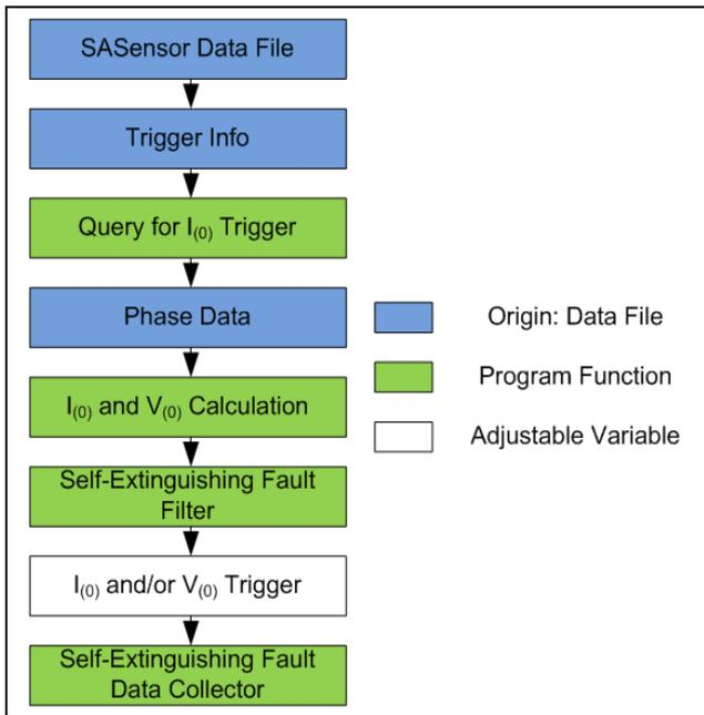
Fig. 16. Processing Scheme of Filtering
