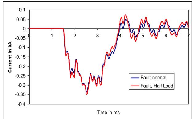
Fig. 12. Simulation of self-extinguishing single phase fault in a network with isolated neutral, fault location 9 km
