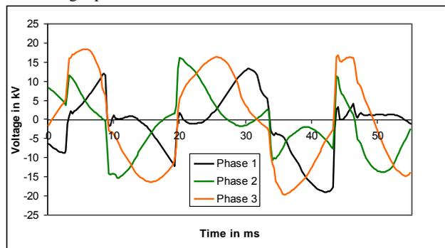
Fig. 3. Measured phase voltages during a self-extinguishing single phase fault in a network with isolated neutral
