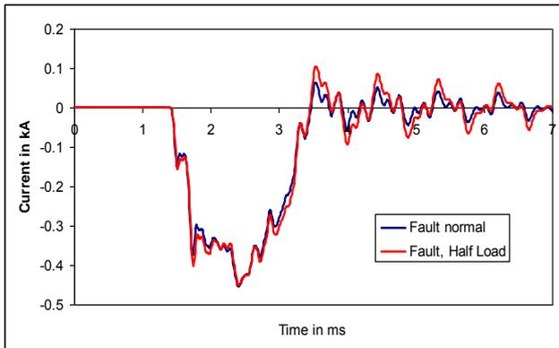
Fig. 11. Simulation of self-extinguishing single phase fault in a network with isolated neutral, fault location 5 km
