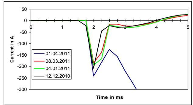
Fig. 8. Different self-extinguishing single phase fault current events at a substation with low-impedance earthing at the same location
