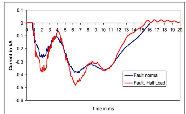
Fig. 14. Simulation of self-extinguishing single phase fault in a network with low-impedance earthing, fault location 5 km
