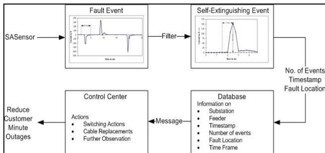
Fig. 1. Idea behind fault prediction in 10 kV MV cable networks
