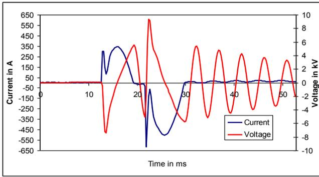
Fig. 7. Zero-sequence current and voltage of a restriking self-extinguishing single phase fault in a network with low-impedance earthing
