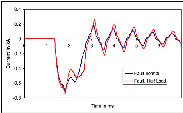
Fig. 10. Simulation of self-extinguishing single phase fault in a network with isolated neutral, fault location 1 km
