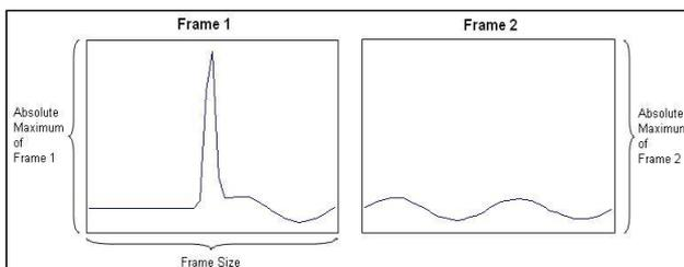
Fig. 17. Maxima frame comparison filter design
