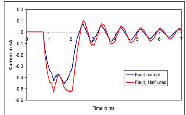
Fig. 13. Simulation of self-extinguishing single phase fault in a network with low-impedance earthing, fault location 1 km
