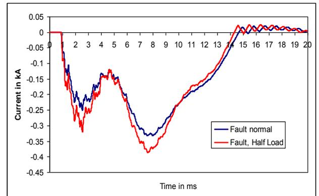
Fig. 15. Simulation of self-extinguishing single phase fault in a network with low-impedance earthing, fault location 9 km
