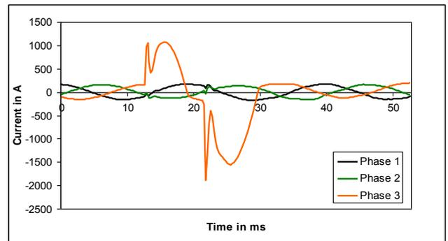
Fig. 5. Measured phase currents during a self-extinguishing single phase fault in a network with low-impedance earthing
