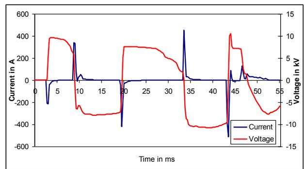
Fig. 4. Zero-sequence current and voltage of a restriking self-extinguishing single phase fault in a network with isolated neutral
