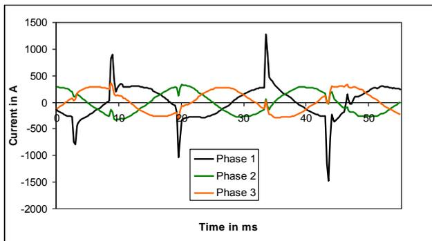
Fig. 2. Measured phase currents during a self-extinguishing single phase fault in a network with isolated neutral
