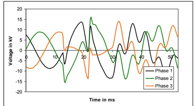
Fig. 6. Measured phase voltages during a self-extinguishing single phase fault in a network with low-impedance earthing
