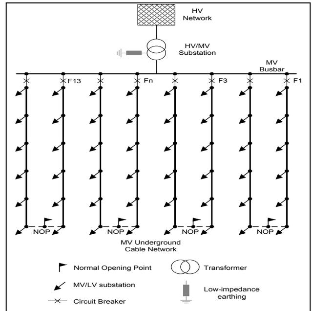
Fig. 9. Typical Alliander 10 kV cable network configuration
