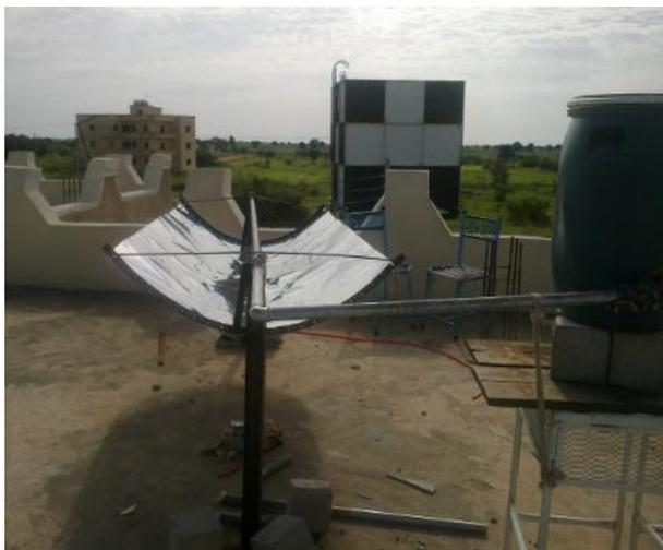
Fig.2 The solar collector setup
