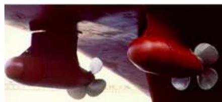
Fig. 6. Simple example of the propeller used in electric propulsion
