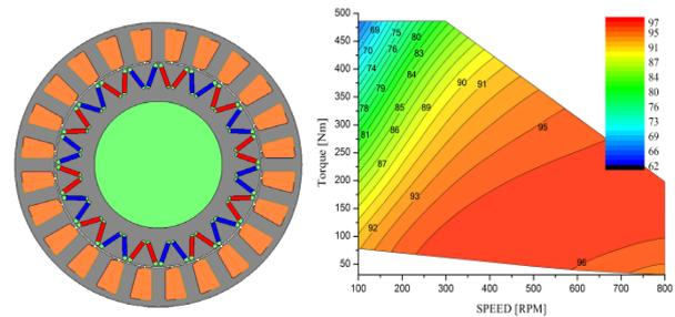
Fig.1 Designed IPM motor and its efficiency map
