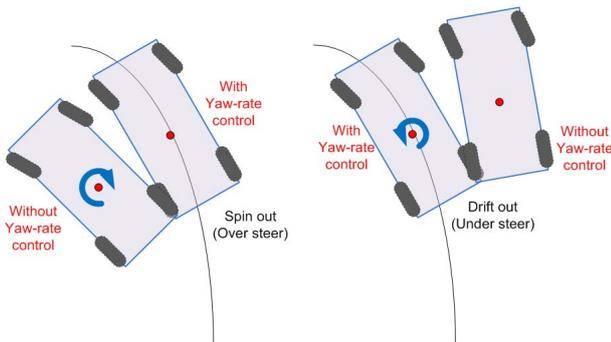
Fig.4 Yaw rate control for over steer and under steer
