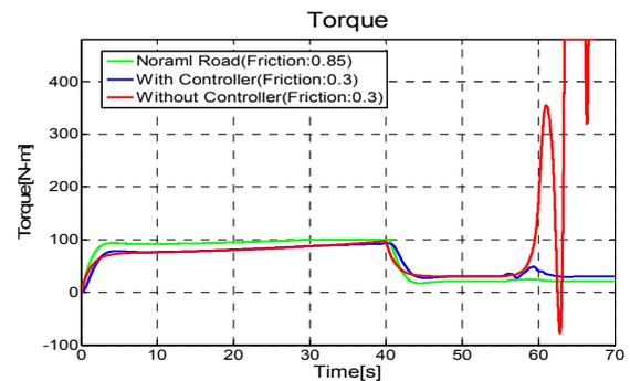
Fig. 10. Simulation result of torque under Double Lane-Change
