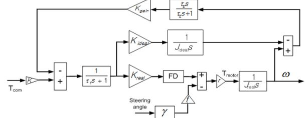
Fig.5 Block diagram of proposed overall algorithm
