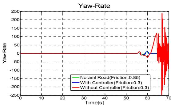
Fig. 8. Simulation result of yaw -rate under Double Lane-Change
