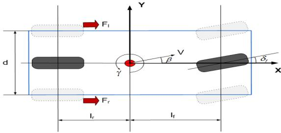
Fig.3 Bicycle model with two degrees of freedom
