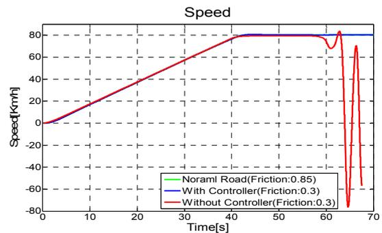
Fig. 11. Simulation result of vehicle speed under Double Lane-Change
