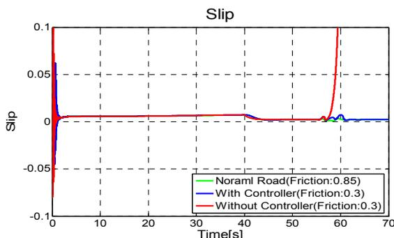
Fig. 9. Simulation result of slip under Double Lane-Change
