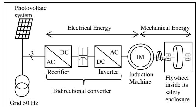
Fig. 6: A FESS connected to the grid and to a photovoltaic system
