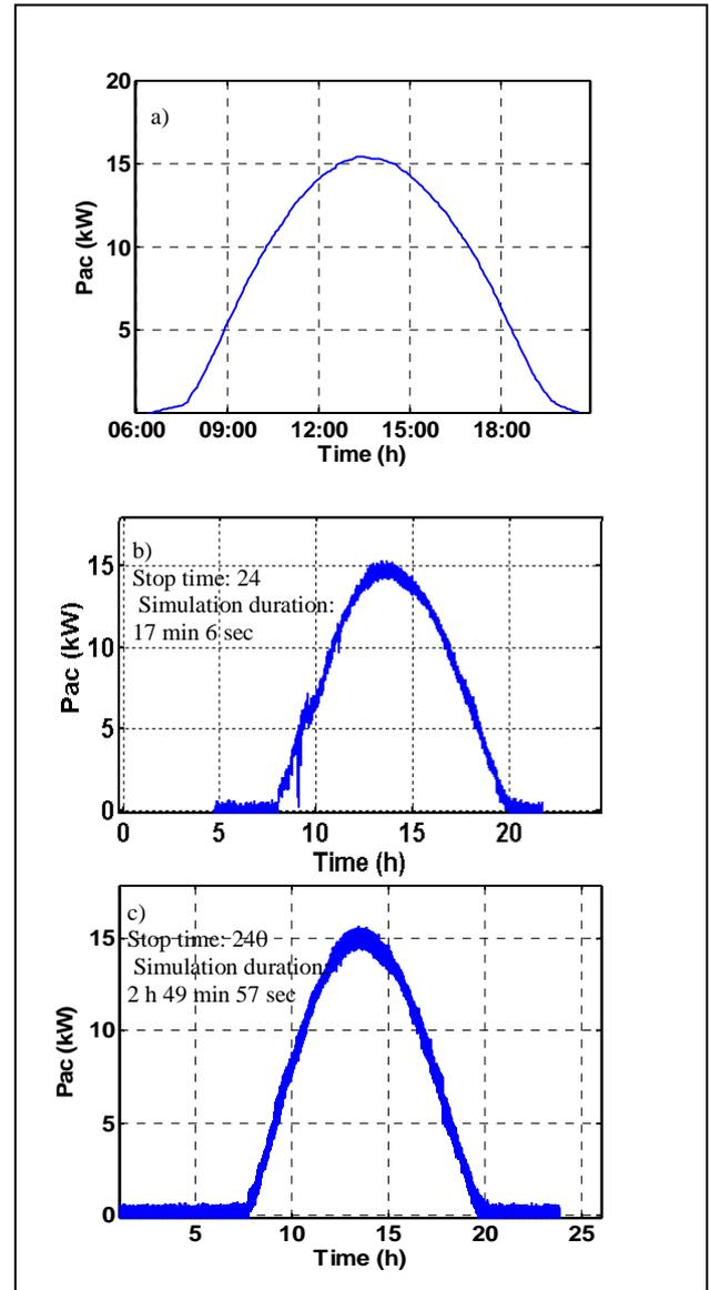
Fig. 3: a) Output of the real 17-kW<sub>AC</sub> Photovoltaic power plant
