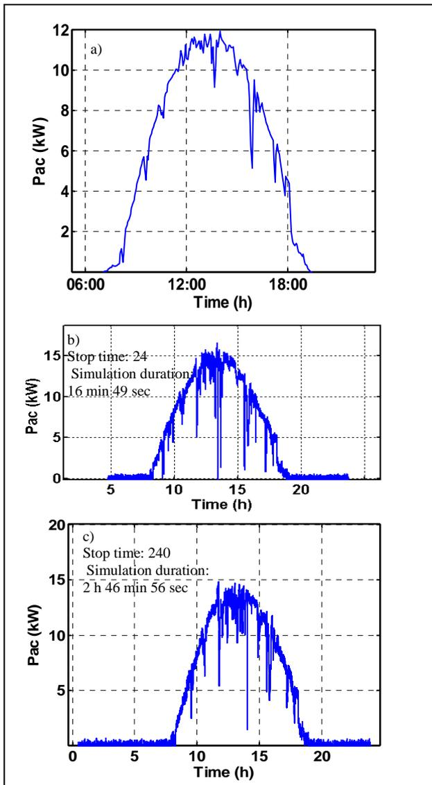
Fig. 4: a) Output of the real 17-kW<sub>AC</sub> Photovoltaic power plant
