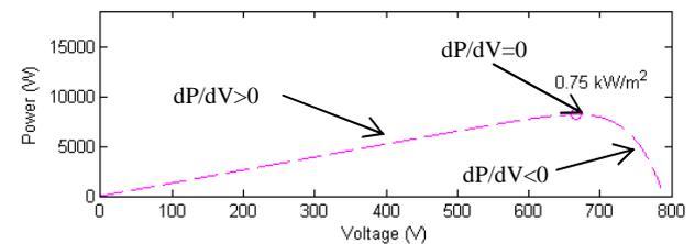
Figure 1: P-V Characteristics at 25°C
