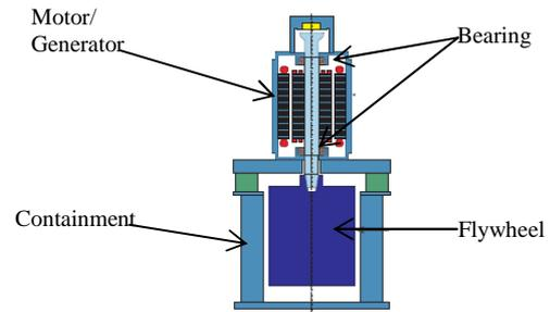
Fig. 5: Basic layout of a flywheel energy storage system [17]
