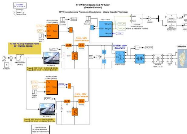
Fig. 2: SimPowerSystems model of the 17-kW Photovoltaic power plant
