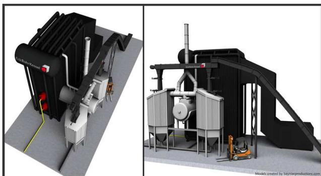
Fig. 3. 3D-Model of twin gasifier, combustor and boiler.
