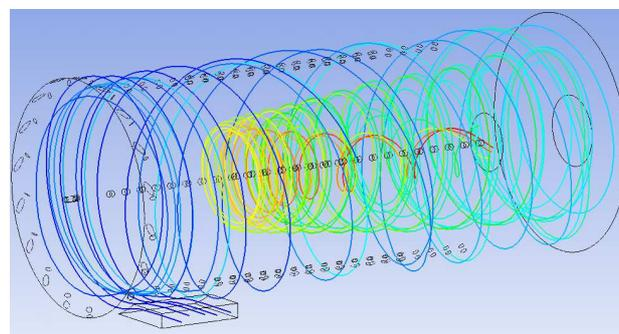
Fig. 6. Resulting streamlines calculated numerically (CFD).
