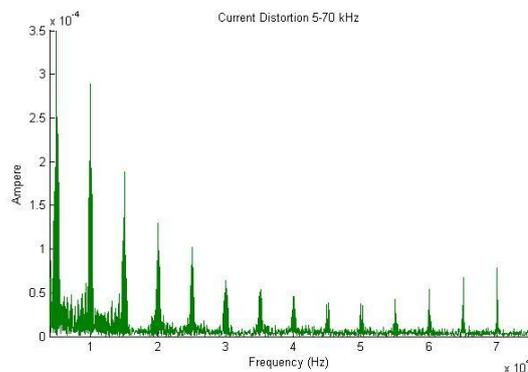
Fig.11. Current distortion generated by charger-A when operated simultaneously
