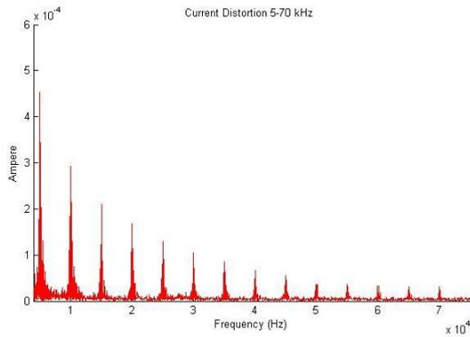
Fig.5. Current distortion generated by CFL-B when operated individually
