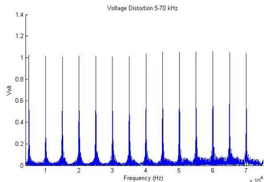
Fig. 3. Voltage distortion level applied to the DUT
