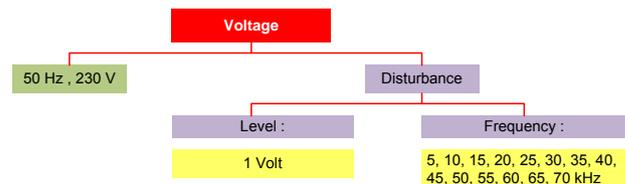
Fig. 2. Voltage Input Distortion Diagram
