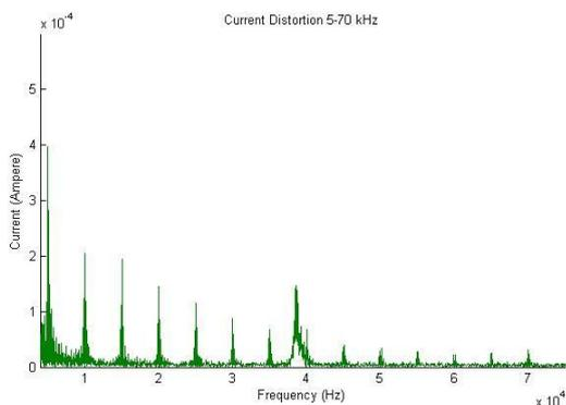
Fig.8. Current distortion generated by CFL-A when operated simultaneously
