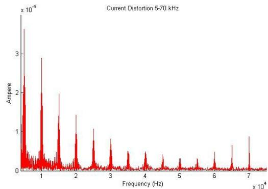
Fig.7. Current distortion generated by Charger-A when operated individually
