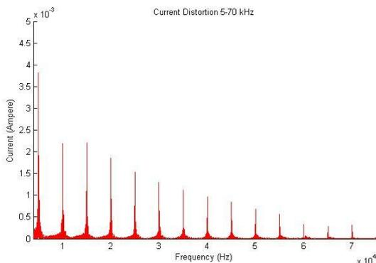
Fig.6. Current distortion generated by LED lamp when operated individually
