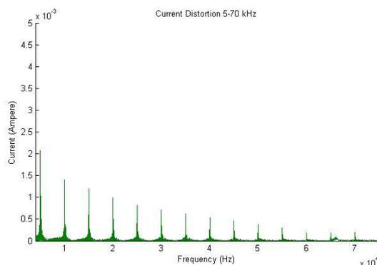
Fig.10. Current distortion generated by LED lamp when operated simultaneously
