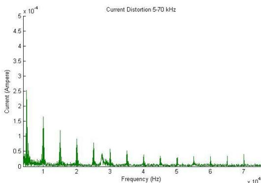
Fig.9. Current distortion generated by CFL-B when operated simultaneously
