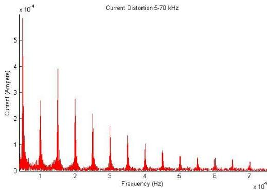
Fig.4. Current distortion generated by CFL-A when operated individually
