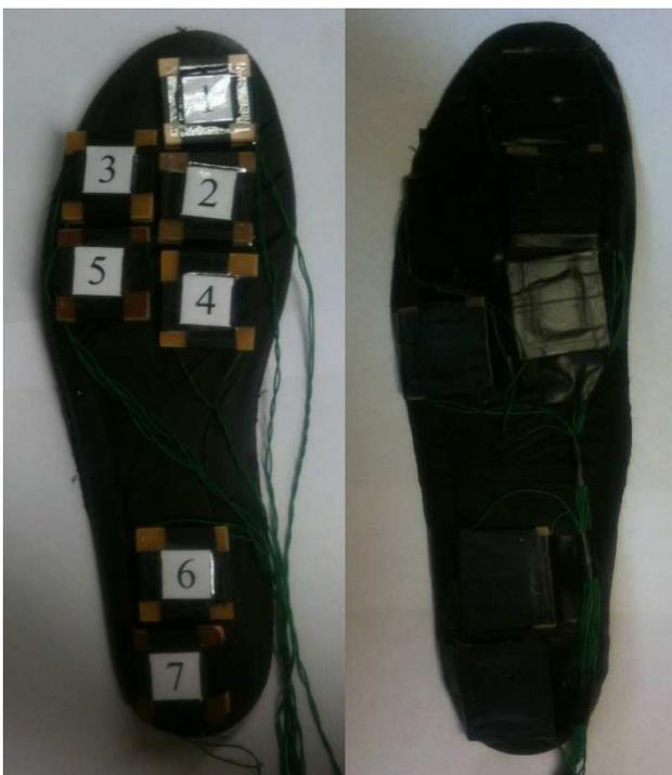
Fig.7: Installation of Piezoelectric Transducers in Footbed.
