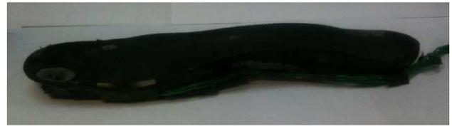
Fig.8: Mounting of Piezoelectric Sensors in Footbed.
