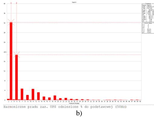
Fig. 11. Voltage and current waveforms when supply a computer unit by means of UPS (Active Power-Model Easy 800 VA) (a); current harmonics spectrum (b).
