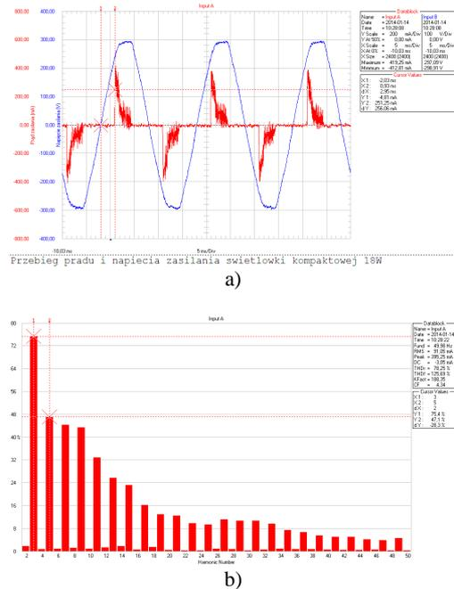
Fig. 4. Voltage and current waveforms for compact fluorescent lamp Brilux 2U 18 W type (a); current harmonics spectrum (b).
