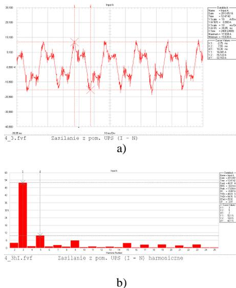
Fig. 13. Current waveform in neutral conductor of a 3-phase low voltage network supplying the server room (a); current harmonics spectrum (b).
