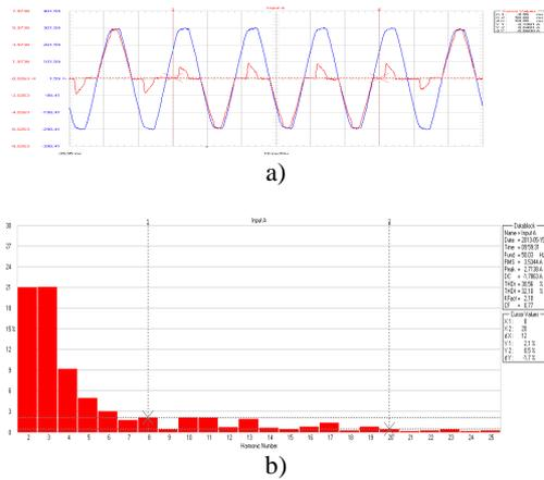
Fig. 8. Voltage and current waveforms when supply printer of HP Laser Jet 2840 type (a); current harmonics spectrum (b).
