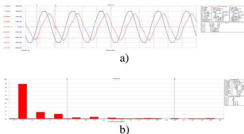
Fig. 3. Voltage and current waveforms for fluorescent lamp LF 2x40 W type (a); current harmonics spectrum (b).
