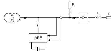
Fig. 14. Simplified electric scheme of system for laboratory testing of operation efficiency of active power filter (APF).
