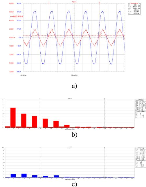
Fig. 1. Voltage and load current waveforms supplied the tested object (a); current harmonics spectrum (b); voltage harmonics spectrum (c).
