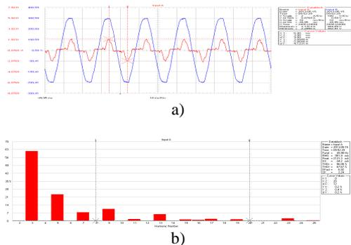
Fig. 10. Voltage and current waveforms when supply a PC kit (computer+monitor+printer) (a); current harmonics spectrum (b).
