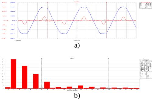
Fig. 9. Voltage and current waveforms when supply scanner of HP Scan Jet 4850 type (a); current harmonics spectrum (b).
