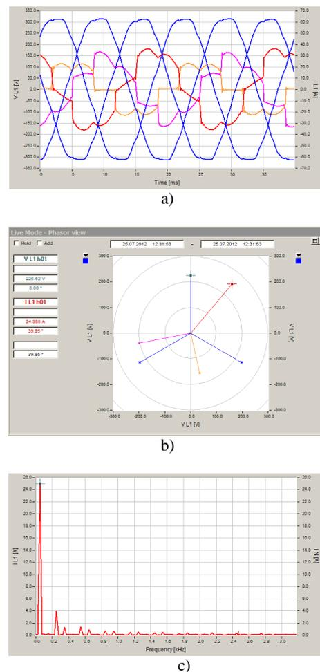
Fig. 15. Current and supply voltage waveforms due to controlled rectifier ( $\alpha=50^\circ$ ) at involved load asymmetry between L1 and L3 phase (a); phase voltage and current vector diagram (b); current harmonics spectrum in L1 phase (c).
