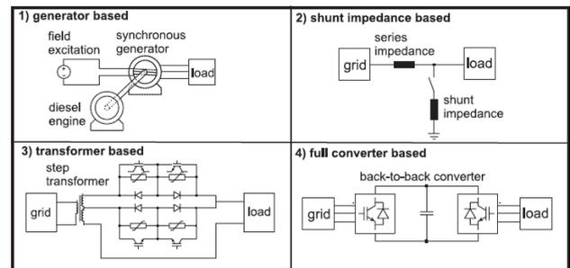
Fig. 1. Voltage dip generator types [6]
