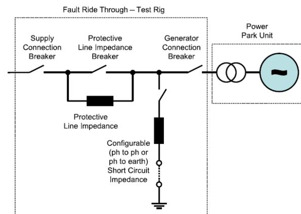
Fig. 3. Low voltage ride-through test circuit used in UK
