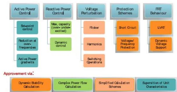
Fig. 4. Grid code requirements and corresponding simulation practices [18]
