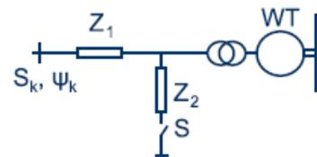
Fig. 2. Low voltage ride-through test equipment principle in IEC61400-21
