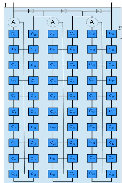
Fig. 2. Circuit model of partially shaded PV module
