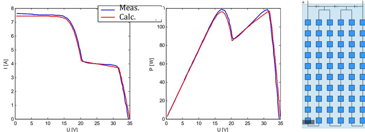
Fig. 3. Measured and calculated current-voltage ( $I-U$ ) and power-voltage ( $P-U$ ) characteristics of the tested PV module for solar irradiance  $G=860 \text{ W/m}^2$  and module temperature  $T=31^\circ\text{C}$  – solar irradiance in the marked solar PV cell is uniformly reduced to  $0.35 G$  due to shading.
