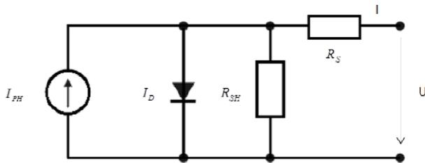
Fig. 1. Single diode solar PV cell model
