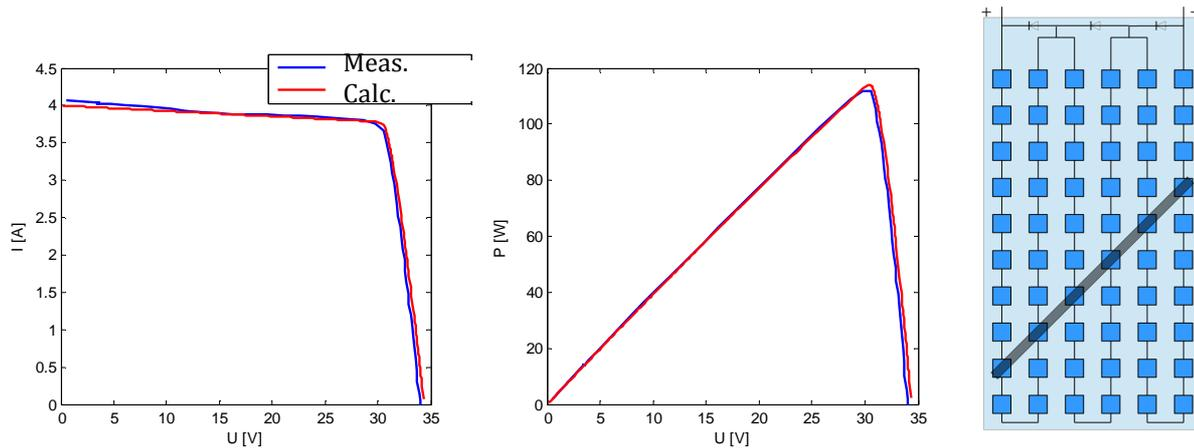
Fig. 5. Measured and calculated current-voltage ( $I-U$ ) and power-voltage ( $P-U$ ) characteristics of the tested PV module for solar irradiance  $G=910 \text{ W/m}^2$  and module temperature  $T=36^\circ\text{C}$  – solar irradiance in the marked solar PV cells is uniformly reduced to  $0.5 G$  due to shading.
