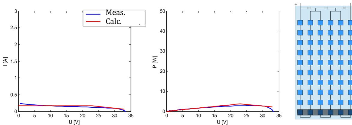
Fig. 6. Measured and calculated current-voltage ( $I-U$ ) and power-voltage ( $P-U$ ) characteristics of the tested PV module for solar irradiance  $G=910 \text{ W/m}^2$  and module temperature  $T=41^\circ\text{C}$  – solar irradiance in the marked PV cell is uniformly reduced to zero due to shading.
