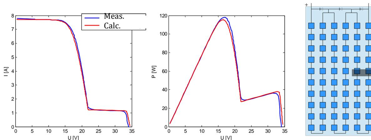
Fig. 4. Measured and calculated current-voltage ( $I-U$ ) and power-voltage ( $P-U$ ) characteristics of the tested PV module for solar irradiance  $G=890 \text{ W/m}^2$  and module temperature  $T=35^\circ\text{C}$  – solar irradiance in the marked solar PV cell is uniformly reduced to  $0.15 G$  due to shading.
