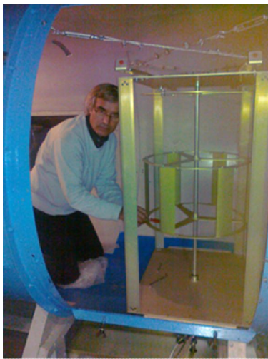
Fig. 1. Schematics of the two stages VAWT experimental model.
