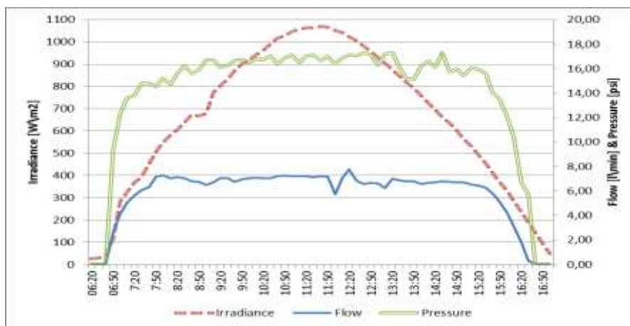
Figure 4: Irradiance, flow and pressure values in a sunny day
