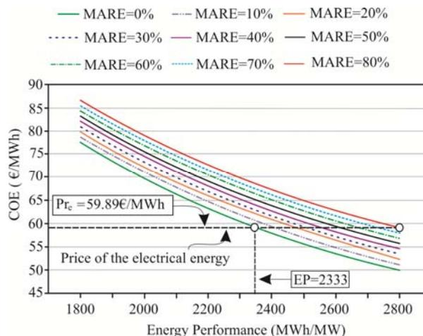
Fig. 3. Total production cost of the electrical energy generated by a wind farm (COE).
