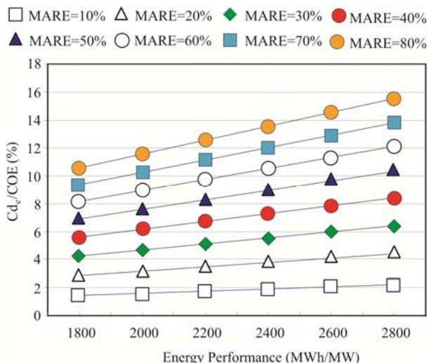
Fig. 2. Contribution of the deviation cost to the production cost of electrical energy by a wind farm.
