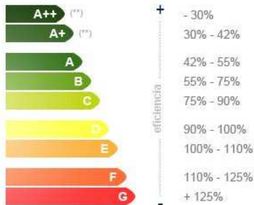
Figure 1. - Energy label and Energy consumption respect to an average consume (E label)
