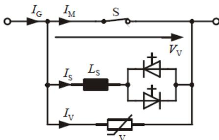
Fig. 1. Conventional Hybrid Circuit Breaker [17].
