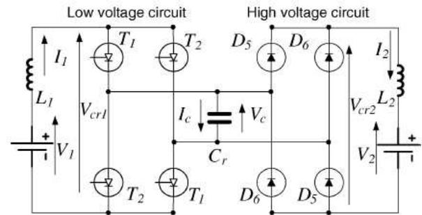
Fig. 2. DC/DC Converter, unidirectional step up converter [19].
