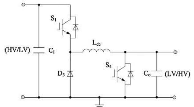
Fig. 3. DC chopper, two-switch topology [20].
