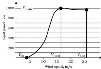
Fig. 2. The wind turbine power curve.
