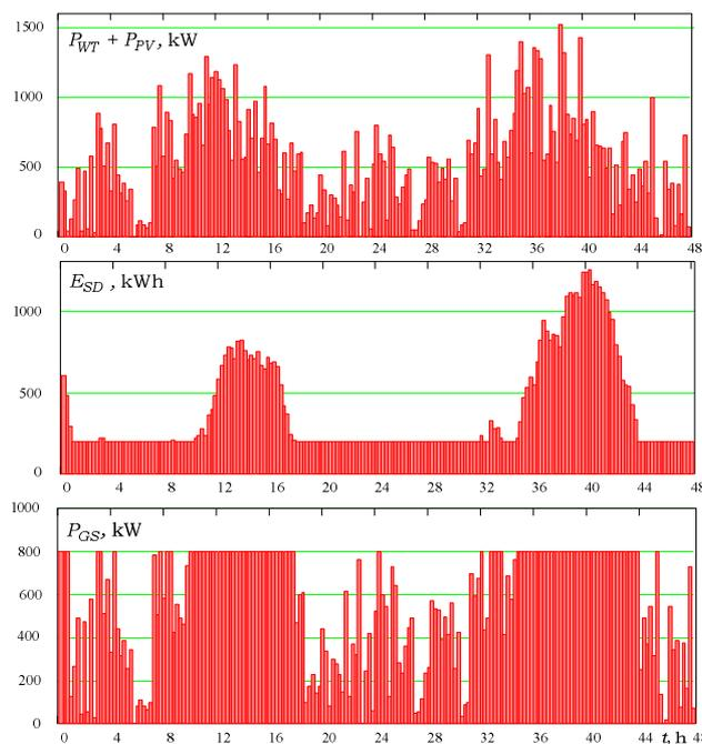
Fig. 8. The microgrid simulated power flows with SD.
