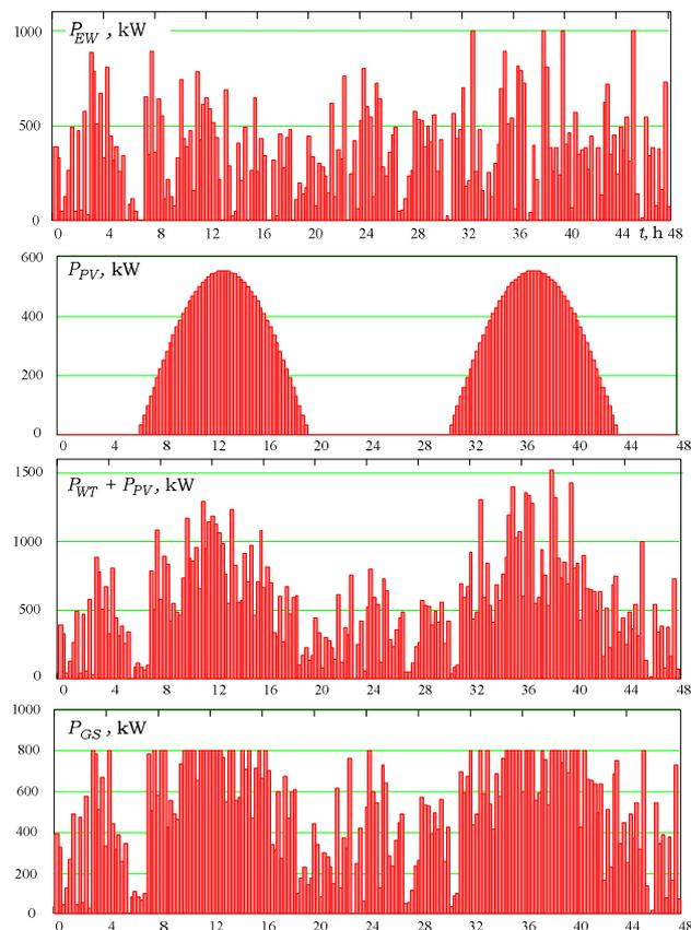
Fig. 7. The microgrid simulated power flows without SD.
