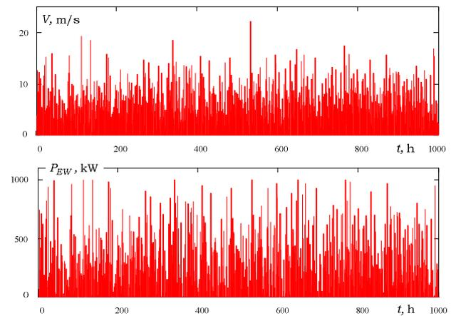
Fig. 4. Simulated wind speed and WT power input time dependencies.
