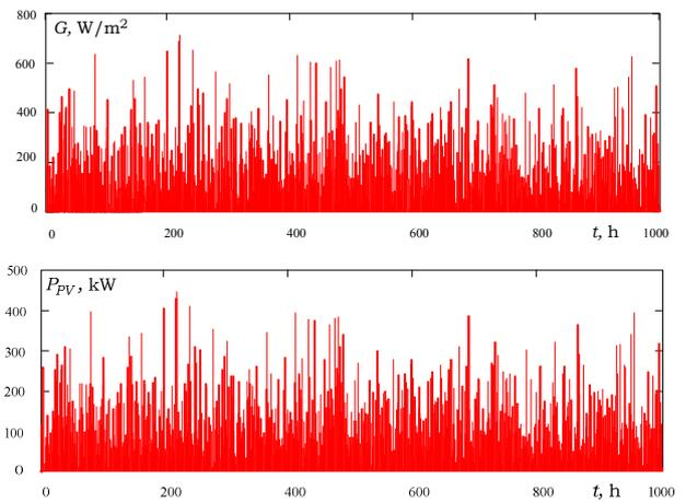
Fig. 6. Simulated solar irradiation and PV power input time dependencies.
