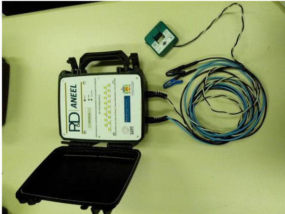
Fig. 5. Photo of the metering device with alligator terminals for tension measurement and with current transformer for current measurement.
