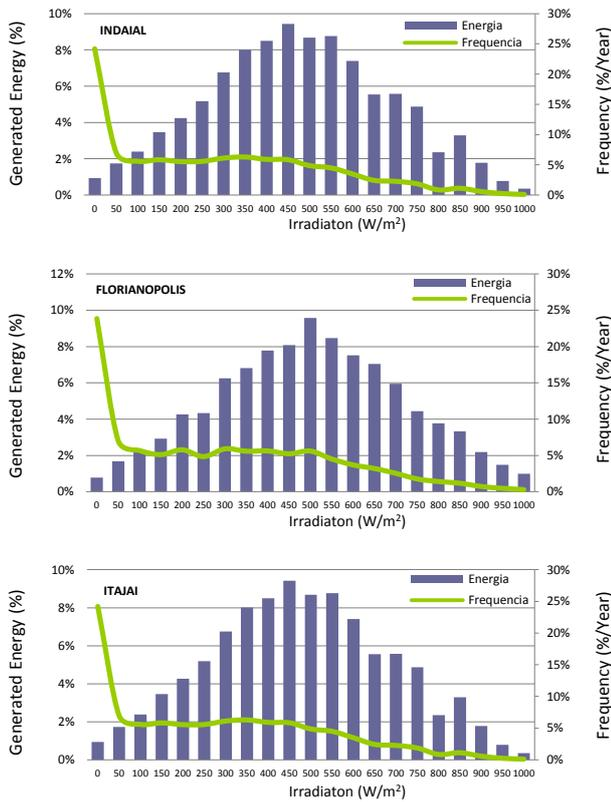
Fig. 2 – Energy available per year for each band of radiation and frequency of occurrence
