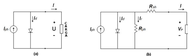
Fig. 1. Equivalent circuit of the solar panel connected to a load: (a) the ideal model and (b) the real model.
