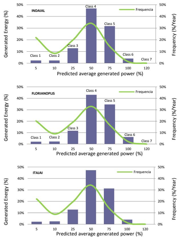
Fig. 3 – Available energy per year as power band established by IEC 61683 for a 245W system in the city of Indaial, Florianópolis and Itajai – Brazil.
