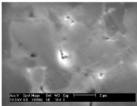
Fig.6. Plan view SEM image of 6H-SiC chemically etched in (22.5M) 2HF/1Na<sub>2</sub>O<sub>2</sub> (0.5M) solution at 25°C - 60 min
