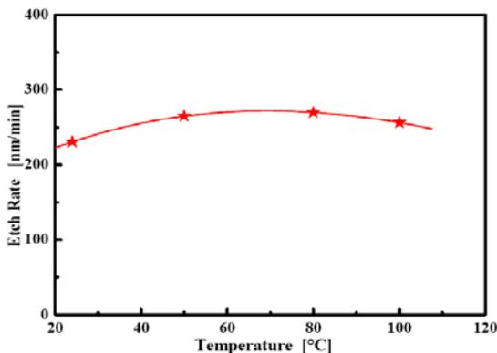
Fig.1. Effect of temperature on the etch rate of 6H-SiC in (22.5M) 2HF/ $1\text{Na}_2\text{O}_2$  (0.5M) solution at  $80^\circ\text{C}$  - 60 min
