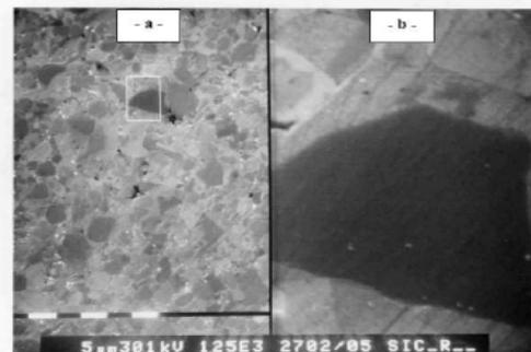
Fig.3. Plan view SEM image of a polished bare 6H-SiC
