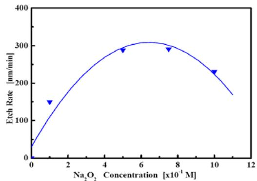
Fig.2. Effect of  $\text{Na}_2\text{O}_2$  concentration on the etch rate of 6H-SiC in (22.5M) 2HF/ $1\text{Na}_2\text{O}_2$  (0.5M) solution at  $80^\circ\text{C}$  - 60 min
