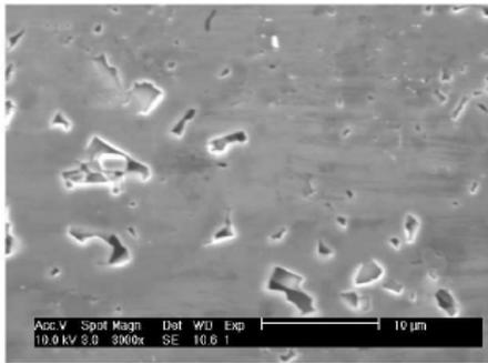
Fig.4. Plan view SEM image of 6H-SiC chemically etched in (22.5M) 2HF/1Na<sub>2</sub>O<sub>2</sub> (0.1M) solution at 80°C - 60 min
