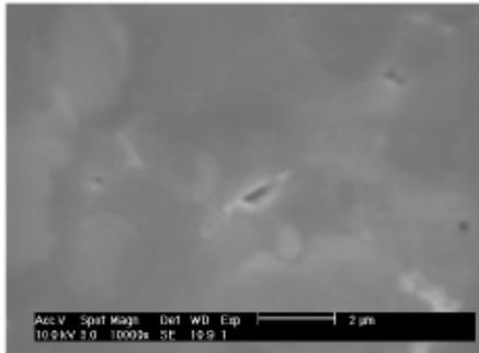
Fig.5. Plan view SEM image of 6H-SiC chemically etched in (22.5M) 2HF/1Na<sub>2</sub>O<sub>2</sub> (0.5M) solution at 80°C - 60 min
