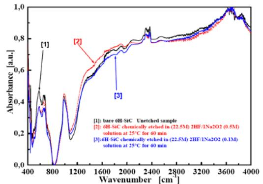
Fig.7. FT-IR Spectra of bare 6H-SiC unetched sample and chemically etched in (22.5M) 2HF/1Na<sub>2</sub>O<sub>2</sub> (0.5M)
