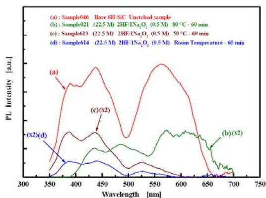
Fig.8. PL spectra of bare 6H-SiC unetched sample and chemically etched in (22.5M) 2HF/1Na<sub>2</sub>O<sub>2</sub> (0.5M)
