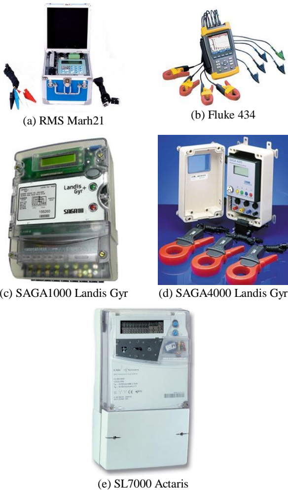
Fig. 1. Measuring equipment used to check the power factor and reactive power flow.
