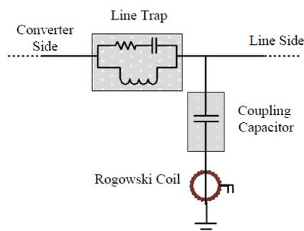
Fig. 1. Travelling wave detection [30]
