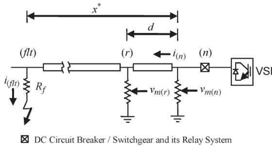
Fig. 4. Distance evaluation with two voltage divider measurements [3]
