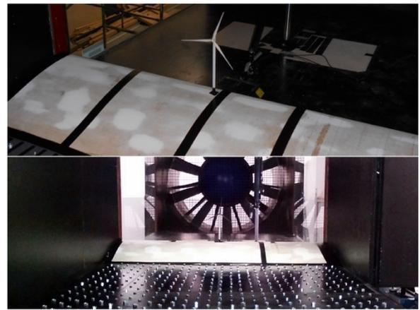
Fig. 2. Hill and wind turbine model placed inside the wind tunnel.
