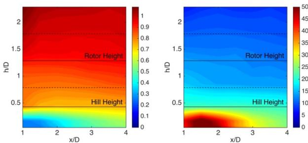
Fig. 5. Mean velocity (left) and turbulence intensity (right) around wind turbine system placed over a hill.
