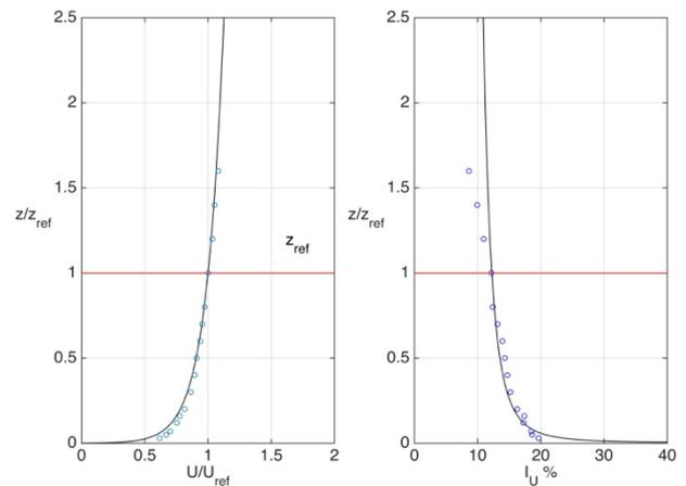
Fig. 3. Theoretical ABL profile (black line) and measured ABL profile (blue circles) for mean velocity (left) and turbulence intensity (right).
