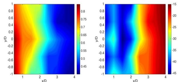
Fig. 8. Top view of mean velocity (left) and turbulence intensity (right) measured at the bottom.
