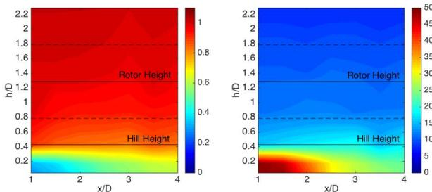
Fig. 4. Mean velocity (left) and turbulence intensity (right) around an isolated hill.
