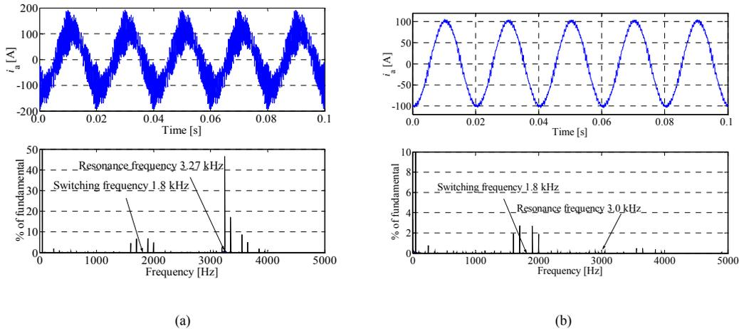
Fig. 4. Phase currents and their frequency spectrums, when  $S_n = 50$  kVA,  $\cos\phi=1$  and  $f_{sw} = 1.8$  kHz. In (a) it can be seen that when the resonance frequency  $f_{res}$  is not carefully selected the line current is very distorted. In (b) both resonance frequencies are carefully placed and the current waveform is much better.
