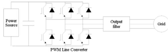
Fig. 1. A typical line converter system in renewable energy applications, where the power is produced by some source to the dc-link and is then rectified and filtered to the grid.
