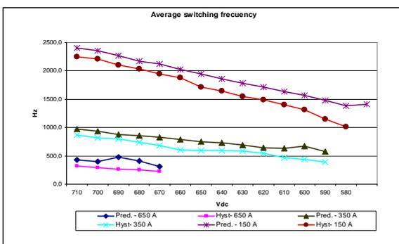
Figure 4. Average switching frequency for traditional and predictive hysteresis controllers.
