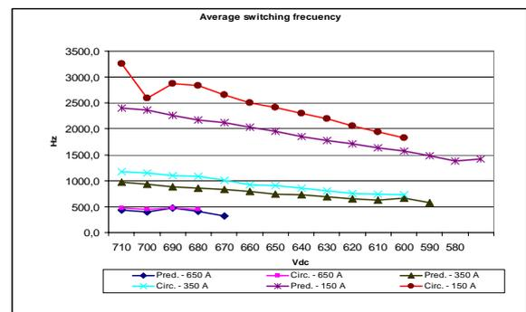
Fig. 7. Average switching frequency for table and predictive circular hysteresis controllers.
