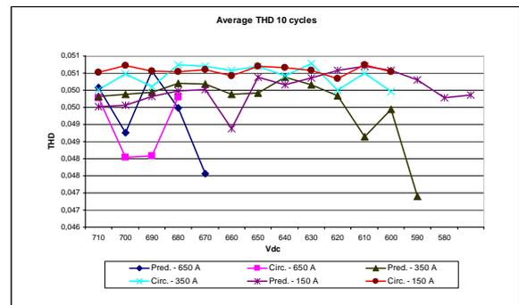
Fig. 6. Average output current THD for table and predictive circular hysteresis controllers.
