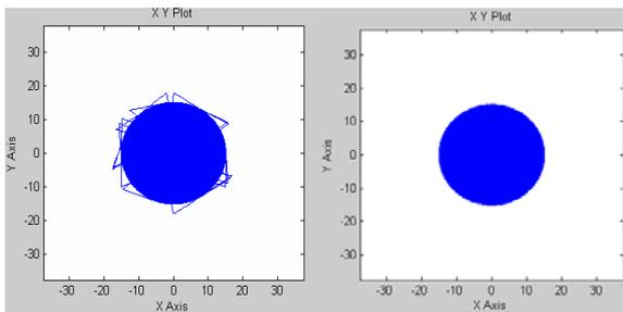
Fig. 8. Error area for table and predictive circular hysteresis controllers.  $I_{out}=150$  A,  $B=15$  A,  $V_{dc}=660$  V.
