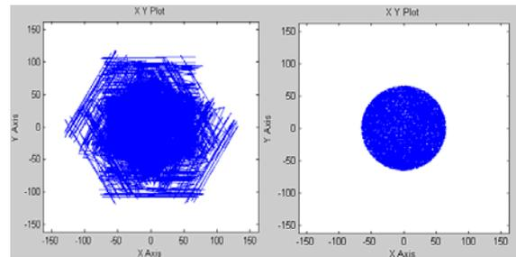
Fig 5. Error area for traditional hysteresis and predictive hysteresis controllers.  $I_{out}=650$  A,  $B=65$  A,  $V_{dc}=700$  V.
