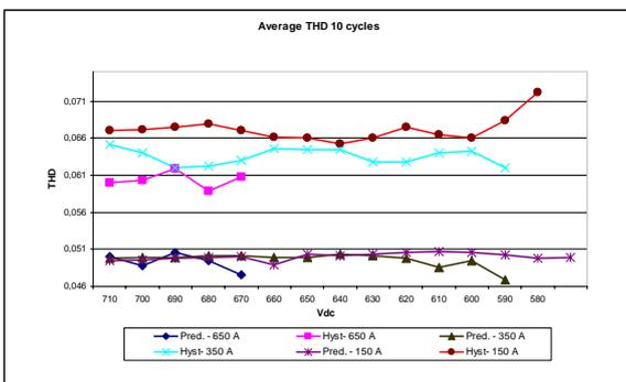
Figure 3. Average output current THD for traditional and predictive hysteresis controllers.
