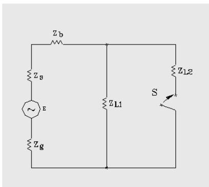
Fig. 7. Supplying two loads with a common source
