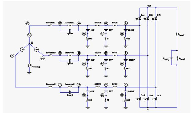
Fig. 15. Circuit diagram of 3-phase PWM controlled rectifier
