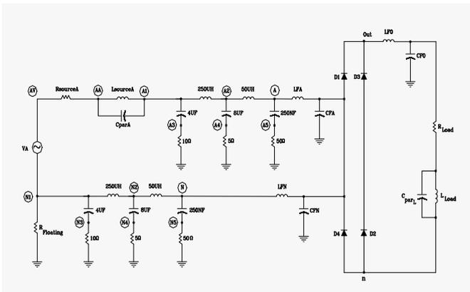
Fig. 3. Circuit diagram of single phase diode rectifier with input and output filters
