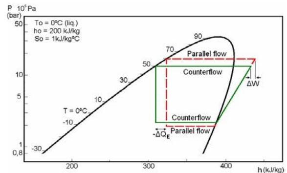
Fig 3. Effects of changing the refrigerant flow direction
