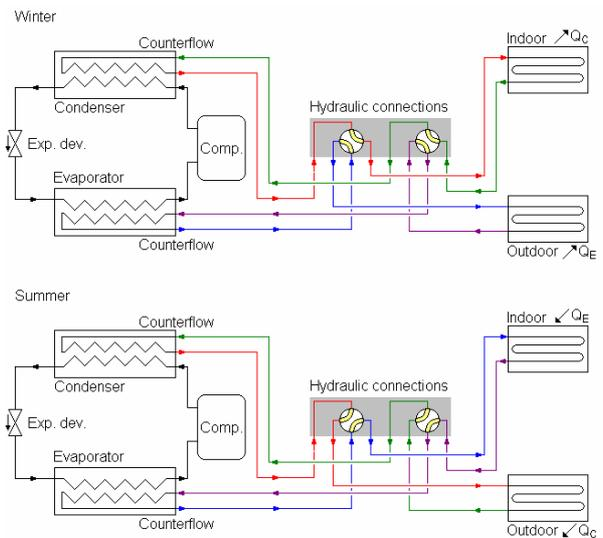
Fig 8. Optimum design with two reversing valves
