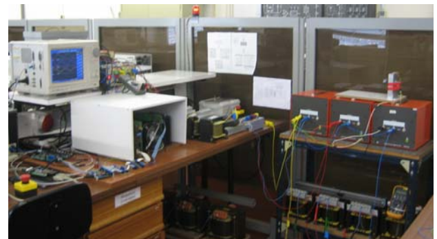
Fig. 2. Laboratory prototype of the Shunt Active Filter.
