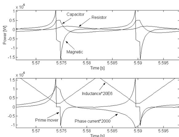
Fig. 12 Non linear case. Upper, instantaneous power in capacitor, load resistor and stored as magnetic. Lower, inductance profile, phase current and instantaneous mechanical power from the prime mover.
