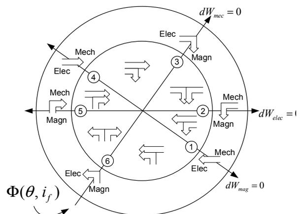
Fig. 6. Trajectories showing the energy flow assuming a linear  $\Phi(\theta, i_f)$  characteristic
