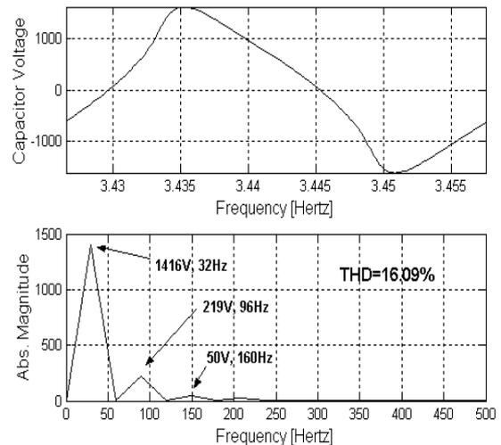
Fig. 13 Harmonic contents of load voltage when saturation is considered. The total harmonic distortion is 16.09% being better than the linear case
