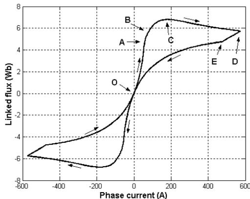
Fig. 8 Phase flux linked versus phase current. Area enclosed represents the energy generated every cycle. The characteristic points A to E are explained in text.
