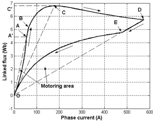
Fig. 9 Detail of characteristic points. Slopes of dashed lines CD and CB represent maximum and minimum of phase inductance.
