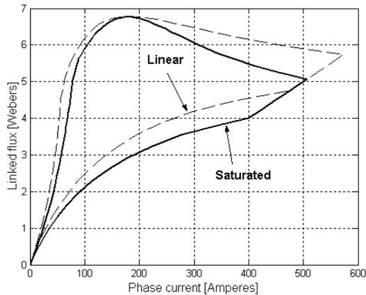
Fig. 11 Comparison of linked flux versus phase current for the linear (dashed) and nonlinear (solid) cases. Capacitor voltage is 1000Vrms in both cases. Saturation reduces the peak current and yields bigger enclosed area.
