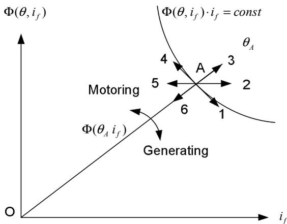
Fig. 5. Directions of six representative trajectories. Trajectories 1 and 2 are generating and 4 and 5 are motoring. Trajectory 3 stores magnetic energy and 6 returns magnetic energy.
