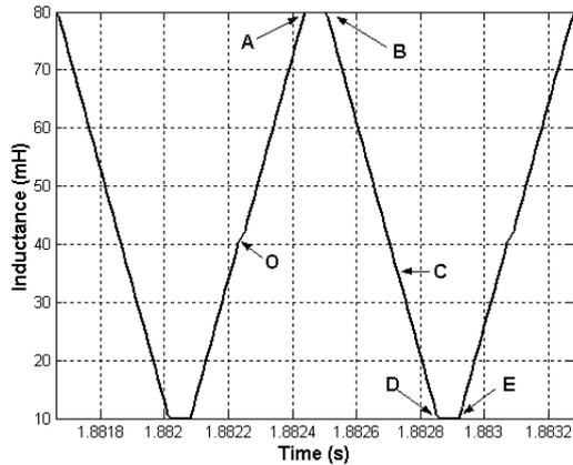
Fig. 7 Hypothetical phase inductance profile with the generator running at 32 turns/s. The characteristic points O to E are explained in text.
