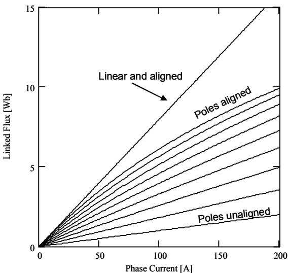
Fig. 10. Nonlinear curves of linked flux versus current using position as parameter and under nonlinear. Upper line is the linear case.
