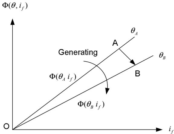
Fig. 4. Clockwise scanned area OAB showing the mechanical energy transformed into magnetic and/or electrical energy.
