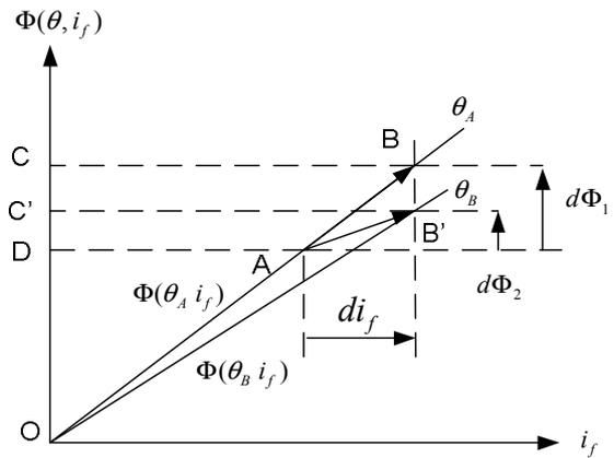
Fig. 3. Trajectory A-B' implies that  $L_f(\theta_A, i_{fA}) \cdot di_f - d\Phi_2 > 0$ . Area OAB' is the mechanical energy supplied to the machine. Area DAB'C' is electrical energy supplied to the machine. Both are stored in the machine as magnetic energy. Trajectory AB implies that  $L_f(\theta_A, i_{fA}) \cdot di_f - d\Phi_2 = 0$ . It only stores electrical energy supplied to the machine as magnetic energy (area DABC).
