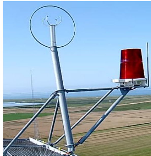
Fig. 8. Anemometer and aviation light LPS.
