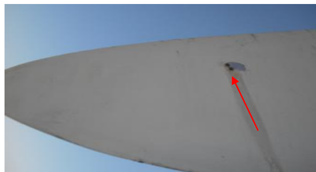
Fig. 2. Lightning hits on blade receptor.
