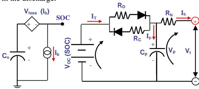
Figure .1. Run-time Battery dynamic Model [4, 6]
