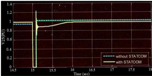
Fig. 20.3: Voltage response of the system at bus-25
