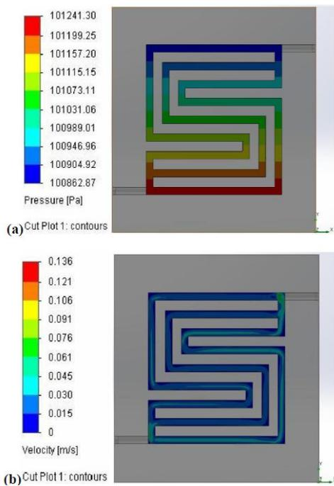
Fig. 3. Water flow simulation with PSFFP (80°C) at the anode side of DE-PEMFC (water flow rate of 12 mL/min at the inlet; environmental pressure at the outlet): (a) Pressure; (b) Velocity.
