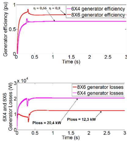
Fig.16. SRG 6/4 and 8/6 (a) Efficiency (b) Losses
