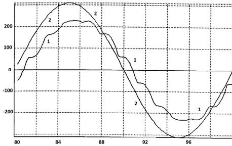
Fig. 6. Waveforms of voltage  $u_{p/2l}$  and current  $i_{R/1l}$  of the supply line, at nominal load of the 2 kW rectifier.
