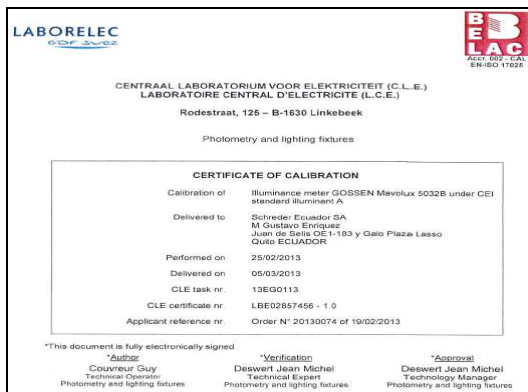
Fig. 2. Calibration certificate for the Mavolux ML 5032B luxmeter
