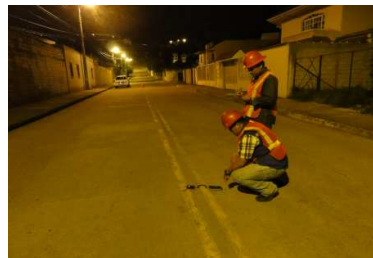
Fig. 4. Performing the illuminance readings at each point of the grid in Araucana street.
