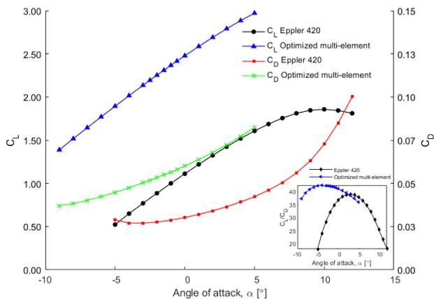
Fig. 6.  $C_L/C_D$  ratio as a function of  $\alpha$  for a traditional hydrofoil and for an optimized multi-element hydrofoil using the Eppler 420 profile.
