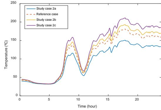
Fig.6. Hot-spot temperature as a function of insulation class.
