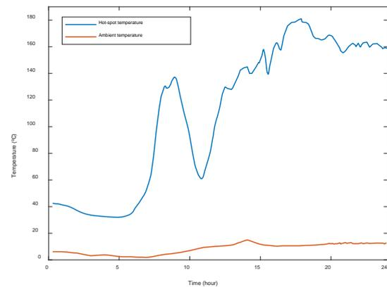
Fig.2. Hot-spot temperature and ambient temperature for the reference study case.
