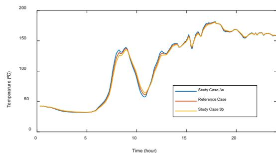
Fig.8. Hot-spot temperature as a function of time constant.
